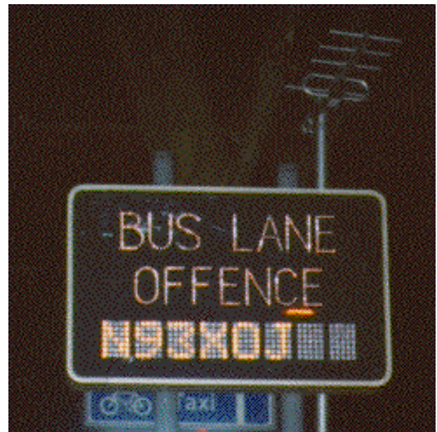
Figure 1 - Variable Message Sign
